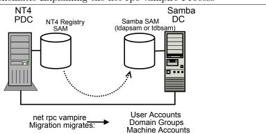
Figure 9.1 Schematic Explaining the net rpc vampire Process
